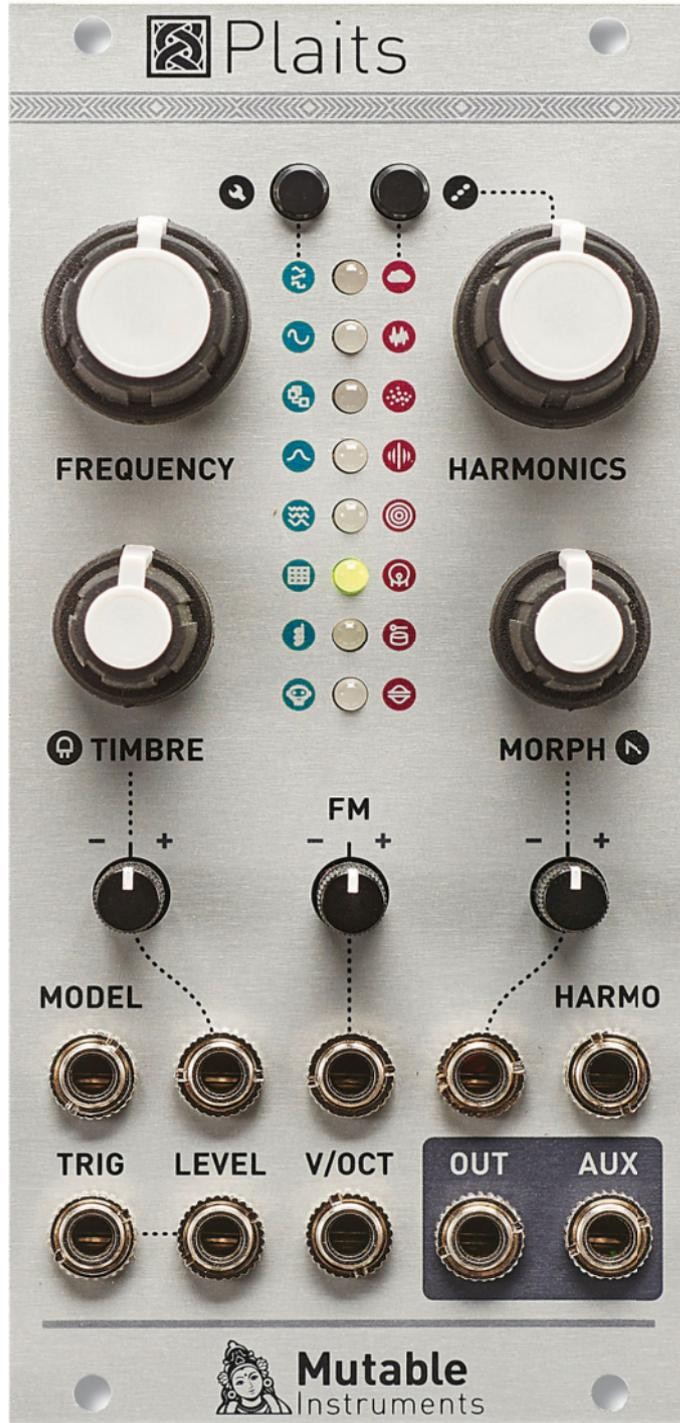
**QUANTISER** Plaits has lost the quantiser from Braids but as most sequencers have built-in quantisers now, it's no issue
