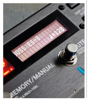
could have one dedicated to amp switching, or one assigned as a tap-tempo switch. A footswitch can be assigned as latching or momentary, so you can trigger an effect for as long as it is held down.
