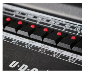
destinations that are simply set via the white and black patch select buttons (press the mod assign button, hit a source, hit a dest, turn the mod amount and watch the LEDs light up across the patch buttons to show level). Or you can directly map many panel controls directly by holding a mod source button and turning a knob/moving a slider. Considering there's no screen it's surprisingly easy to set up and cleverly implemented.
