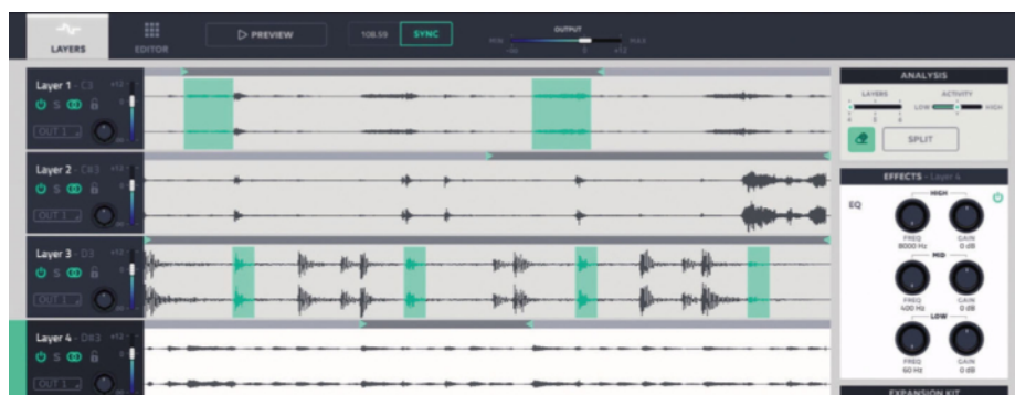
Mark out regions to be moved between Layers using the misleadingly named Annotation tool
