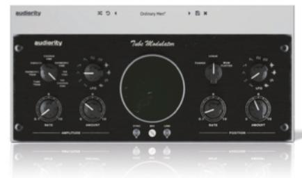
the green dot in the central display moving to reflect both on the Y and X axes. The modelled circuits include various flavours of tremolo, vibrato and chorus on the left, and auto-Panner, Leslie and Wow/Flutter on the right. The speed (sync'd or free from 0.1-10Hz), LFO waveform and amounts of the two modulators are adjusted independently or linked.
