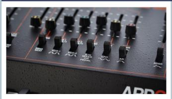
It's great having punchy ADSR and AR envelopes and either can be assigned to the filter or VCA. The LFO has sine and square waves and, while it doesn't run into the audio range (and there's no MIDI sync), it can be assigned to the pitch of both VCOs for vibrato, to the filter and to Sample/Hold for more random/evolving sounds/ FX - note that it has a red rate LED buried in the LFO slider channel too.
