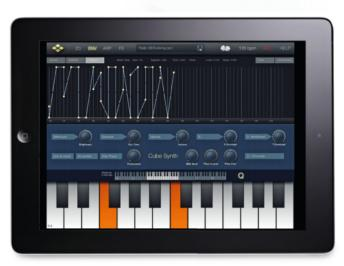
Cube's four-voice morphing setup is its headline feature, fuelling mind-blowingly organic, evolving tones over which extensive control is given to the user. It doesn't hurt that it just sounds superb generally, either, of course.
