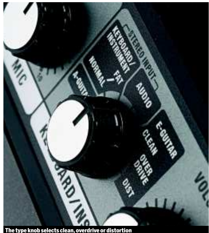
The type knob selects clean, overdrive or distortion
