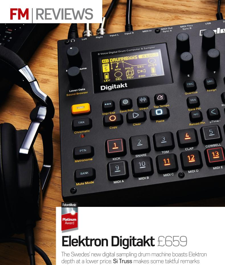
CONTACT who: Elektron web: www.elektron.se KEY FEATURES Standalone sampling drum machine with built-in sequencer. Features eight sample tracks and eight MIDI tracks for external sequencing. I/O: 2x 1/4-inch jack in, 2x 1/4-inch jack main outs, 1x 1/4-inch jack headphone out, MIDI In, MIDI Out, MIDI Thru, USB (for computer/Overbridge connection) DIMENSIONS: 215x176x63mm WEIGHT: 1.45kg
