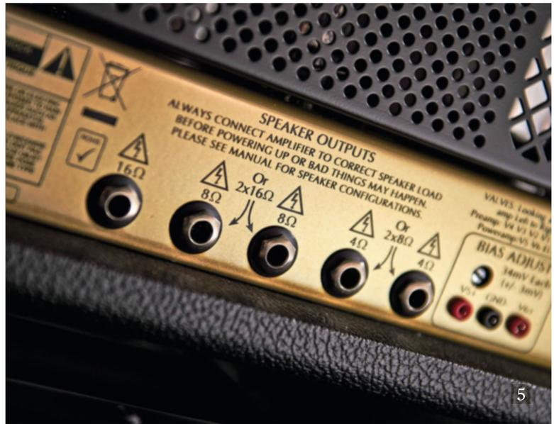
5. The Sheriff 44 offers a comprehensive set of speaker outlets, and its bias switch gives you a choice of fixed or cathode bias modes, which have an effect on output power and power stage response
