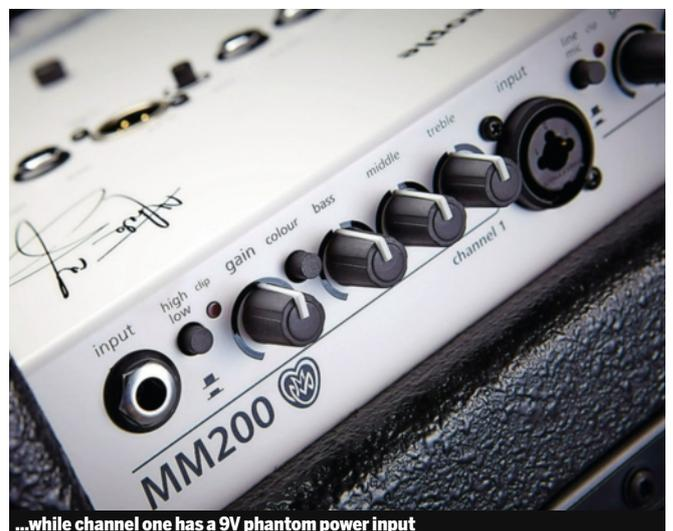
...while channel one has a 9V phantom power input
