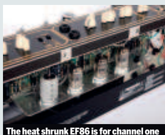
The heat shrunk EF86 is for channel one
