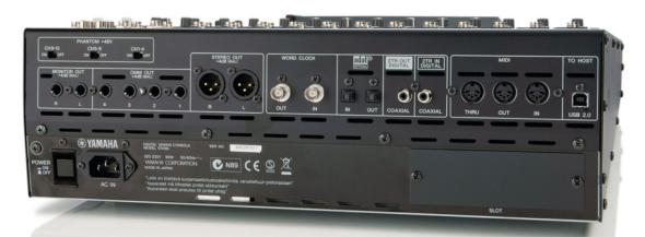
Thru ports and a USB 2.0 connector, of which more shortly. Be aware that despite the proliferation of buttons on the upper surface, the 01V96i remains a console which requires regular menu-diving to set up and operate. Unlike analogue consoles with dedicated EQs, auxes and pan controls, all of these options and more are accessed here via software.
