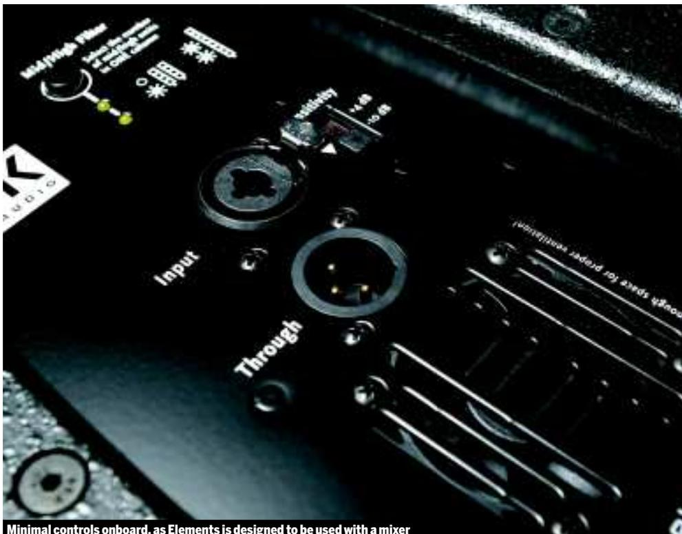
Minimal controls onboard, as Elements is designed to be used with a mixer
