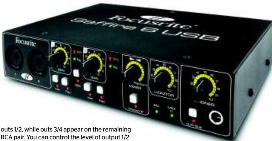
outs 1/2, while outs 3/4 appear on the remaining RCA pair. You can control the level of output 1/2 with the Monitor knob on the front; output 3/4 always comes out at full level.
