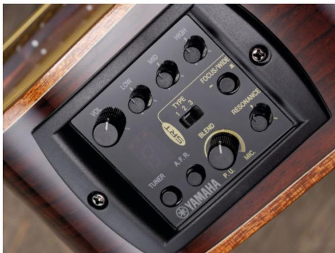
Both 1200s have the ART pickup and SRT preamp system with three-band EQ
