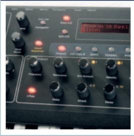
The Prophet 08 features a useful arpeggiator and a versatile 16-step 4-track gated sequencer. The arpeggiator has four modes (up, down, up/down and assign). Its clock can be sync'd with MIDI and has several beat division options ranging from half-note through eighth note swing, up to 64th note triplets if you so desire!
