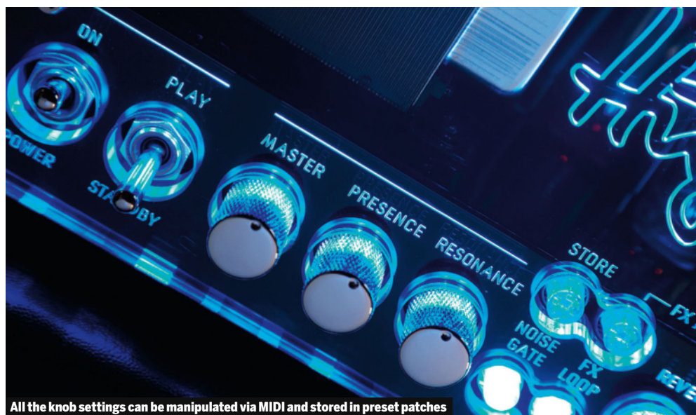
All the knob settings can be manipulated via MIDI and stored in preset patches
