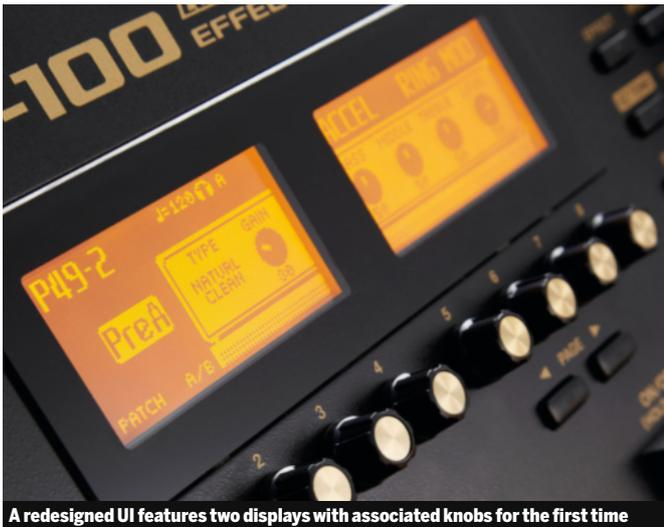
A redesigned UI features two displays with associated knobs for the first time
