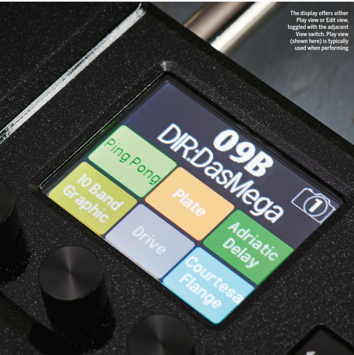
The display offers either Play view or Edit view, toggled with the adjacent View switch. Play view (shown here) is typically used when performing
