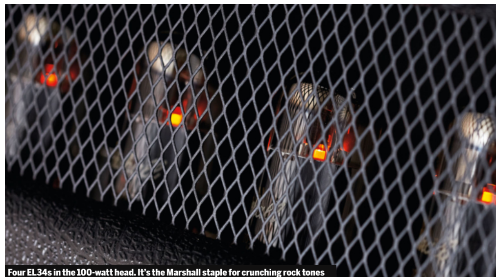
Four EL34s in the 100-watt head. It's the Marshall staple for crunching rock tones
