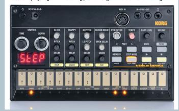
have a MIDI CC and can be addressed via a MIDI controller. For example, you can control filter cutoff (though not resonance) and delay time on the Keys, the hi-hat 'grain', 'stutter' and tom decay on the Beats and gate/ slide time and VCO pitches on the Bass, (though unfortunately not filter cutoff or resonance which I presume is to keep the filter sweeps smooth).
