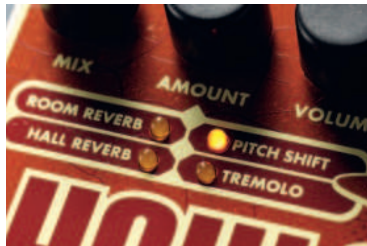
The Holy Stain includes four digital effects: two reverbs, pitch shift and tremolo
