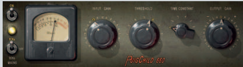
The PuigChild 670 models the ‘variable mu’ effects of a real, valve-based Fairchild compressor
