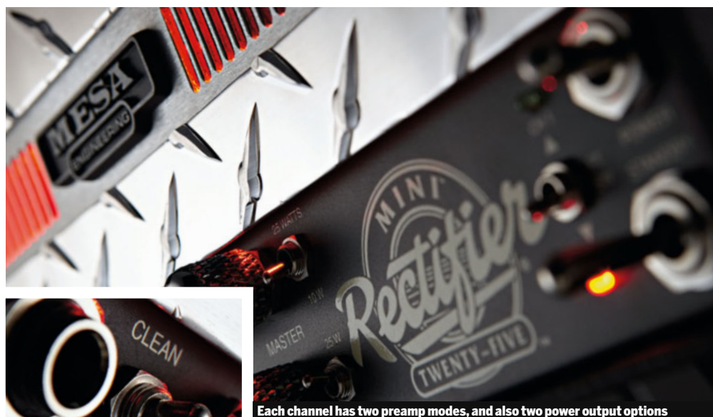
Each channel has two preamp modes, and also two power output options
