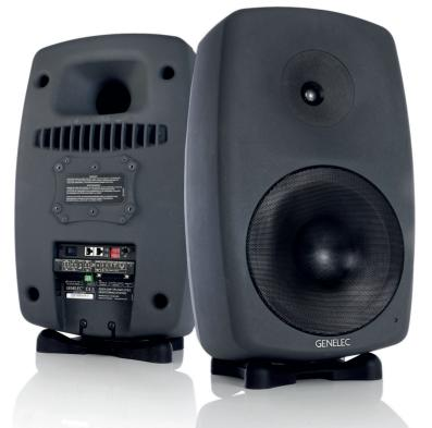
Genelec's own minimum diffraction coaxial mid/hi driver (MDC) which gives a very even and extremely accurate on and off axis response. They can be fed with a digital (AES) or analogue input via XLRs and the DSP section is controlled by connecting a computer with the GLM (Genelec Loudspeaker Manager) software installed, via the CAT5 ports on the back.
