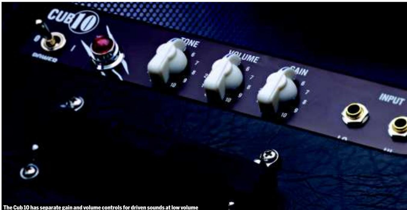
The Cub 10 has separate gain and volume controls for driven sounds at low volume
