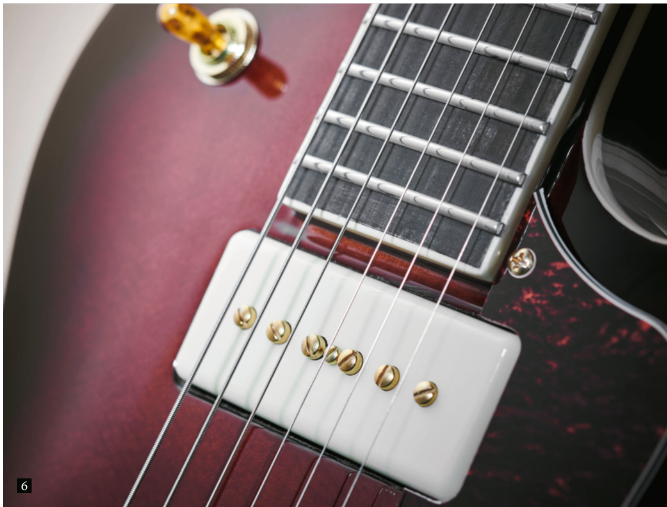
6. These Franz soapbar single coils mount to the guitar in a different fashion to a regular Gibson P-90 (see Under The Hood on the previous page)
