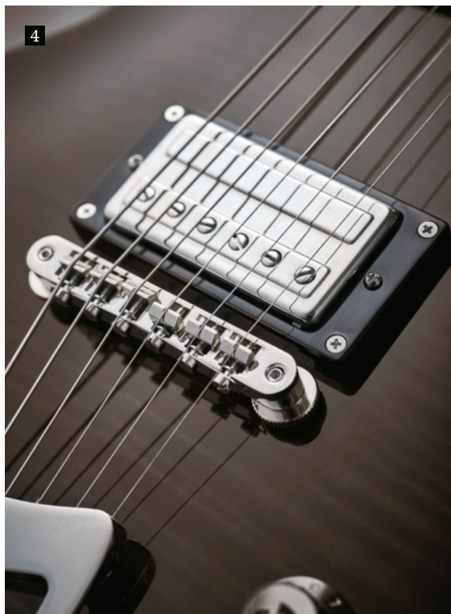
4 & 5. Unlike the existing M-75 Aristocrat, both tune-o-matic bridges here mount directly into the top. The only difference is the gold-plating of the P90 model's bridge (below)
