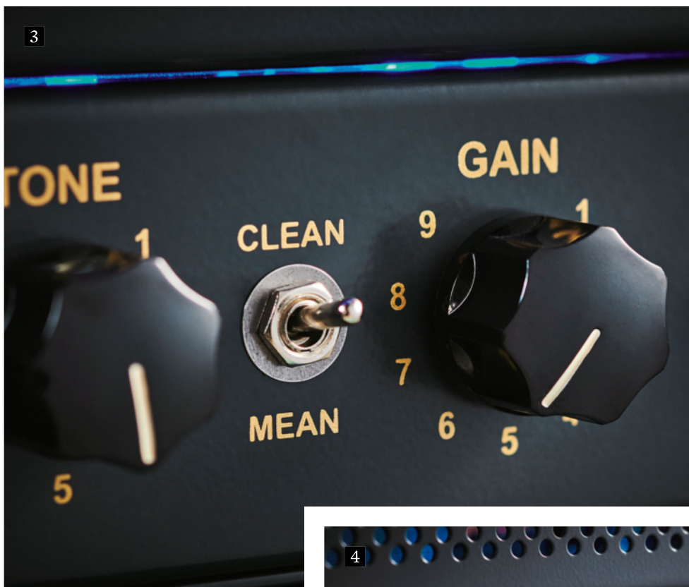
3. The preamp has a Clean/Mean gain switch that flips from clean to a punchy midrange boost
