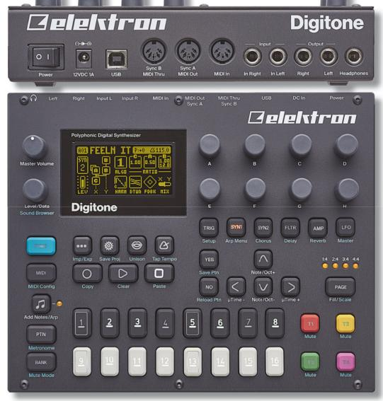
FM ENGINE: A four-operator, eight-algorithm affair with plenty of tweakable parameters
