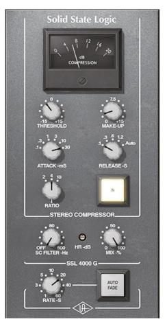
(useful on string or drum groups, for instance) as well as a sidechain filter and a Headroom control too. Elsewhere, the feature set will be familiar to many, with the characteristic grey livery providing Threshold, Attack, Release and Make-Up Gain controls around a choice of 2:1, 4:1 or 10:1 Ratios. The sound is sumptuous; a notable improvement upon its predecessor.
