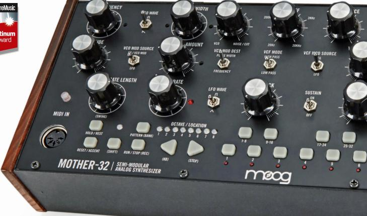
toggle), and can be piloted with the Frequency, Pulse Width and VCO Mod Amount knobs. There's a Glide (portamento) control knob, while the Tempo/Gate Length control below that manages the speed of the sequencer.
