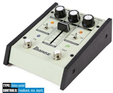
delay time, oscillation switch,
