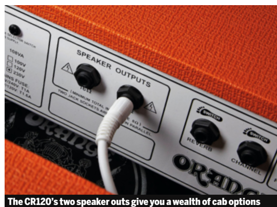
The CR120's two speaker outs give you a wealth of cab options
