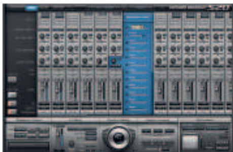
When you touch the Bleed control, a further strip full of levels pops up, enabling mic-by-mic level adjustment
