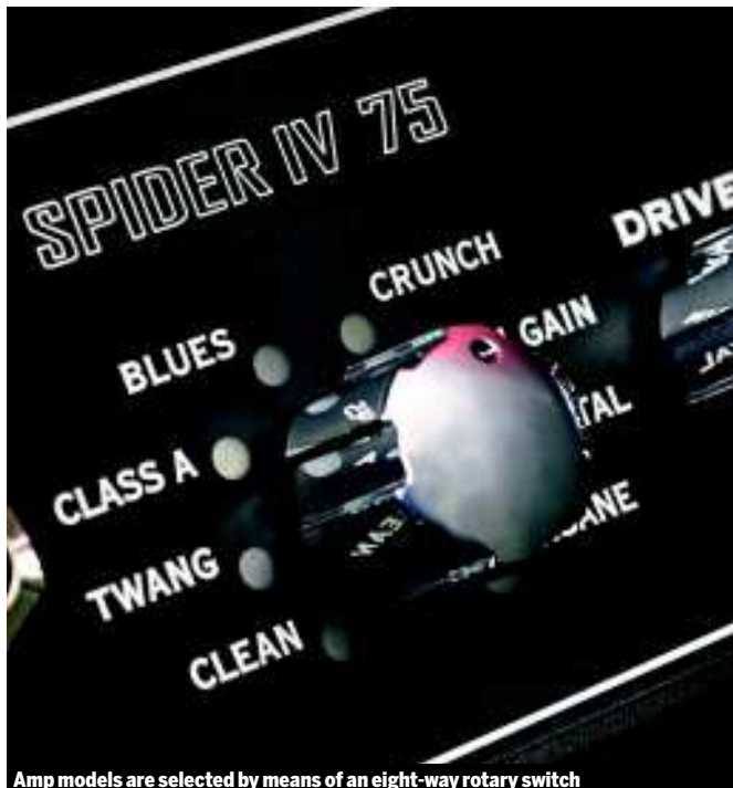
Amp models are selected by means of an eight-way rotary switch
