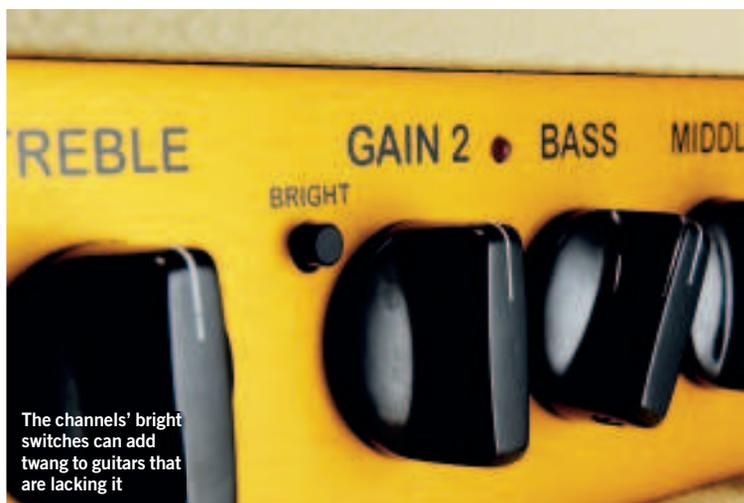
The channels' bright switches can add twang to guitars that are lacking it
