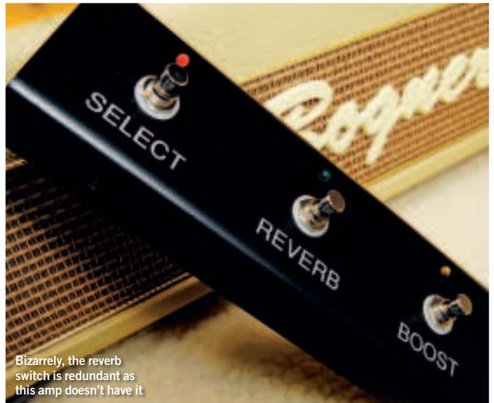
Bizarrely, the reverb switch is redundant as this amp doesn't have it
