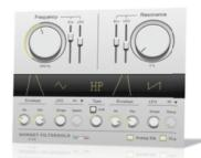
the depths of all four assignments set by the sliders. The LFOs offer four waveshapes and can be synced to host tempo (1/16 to 1 bar) or run free, while the envelope Attack and Release times range from 10-1000ms. The sloping Attack/Release graphic in the main display is quite cool, but we'd prefer to see actual time values as well.
