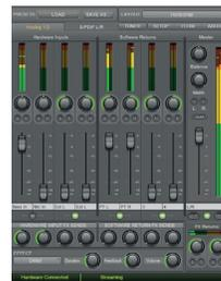
the Mbox and Mbox Pro. The driver control panel includes a mixer of all available paths, both playback and input
