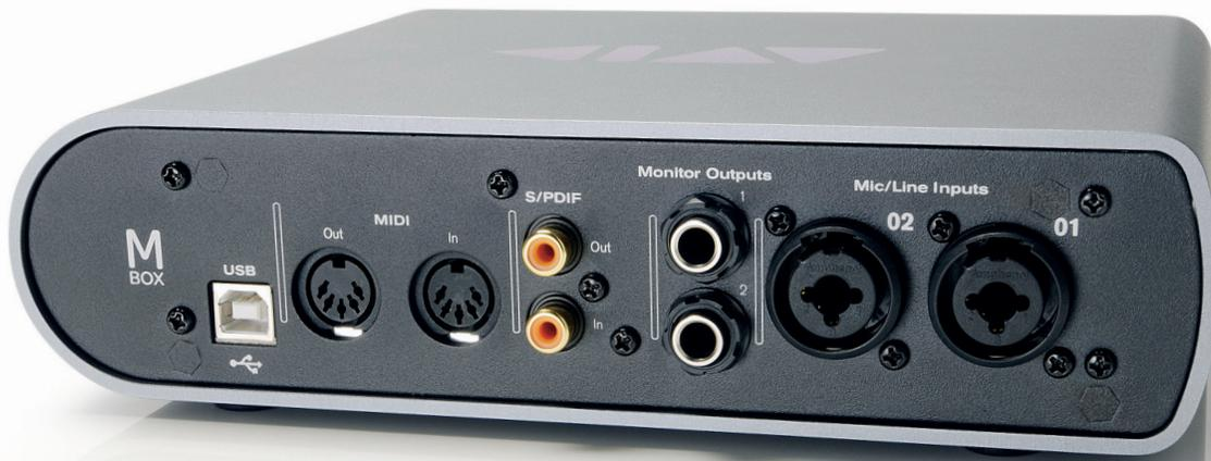
plugging in guitars and it's clear that they've thought hard about practicality and effectively with minimum compromises to keep the price and size down. There are two independent stereo outputs: one analogue and one digital with the analogue output is available for speakers and headphones
