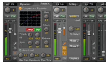
mixes though their quality and range is surpassed by native DAW plugs. The EQ and dynamics offer more quality and make handy tools for monitor mixes during tracking and on send/return paths to external effects. The EQ and dynamics can be
