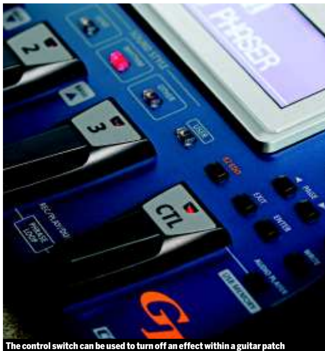
The control switch can be used to turn off an effect within a guitar patch
