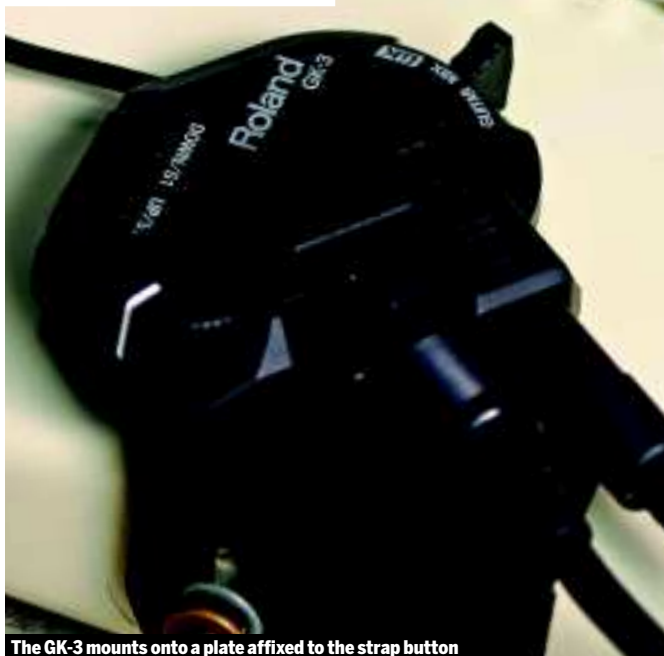
The GK-3 mounts onto a plate affixed to the strap button
