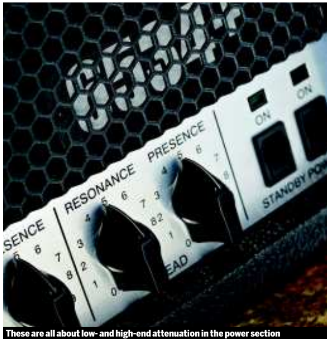
These are all about low- and high-end attenuation in the power section
