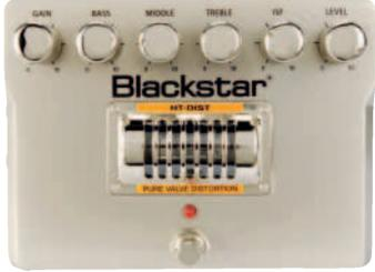
offers a more traditional front panel layout than that offered by the HT-Dual. Like all the pedals on test, the bombproof casing, high quality pots screwed to the chassis, heavy duty switches and high quality jacks all inspire confidence. This is true on the inside too: decent quality components and custom PCB designs, all held in place securely, suggesting a long and happy life.
