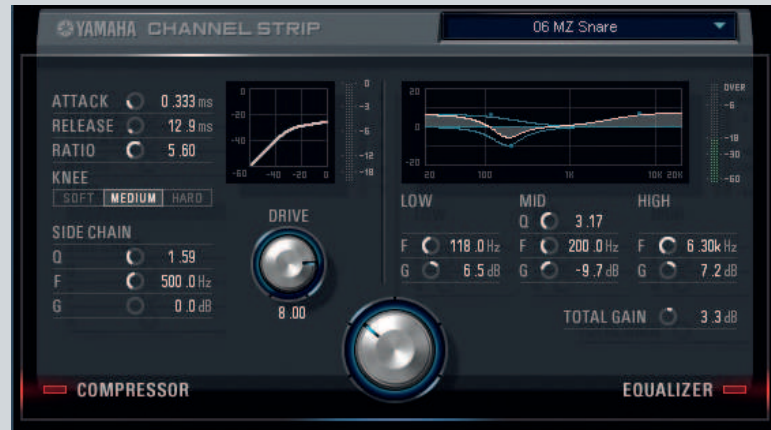
The Channel Strip plug-in offers compression and equalisation with a fairly simple control set
