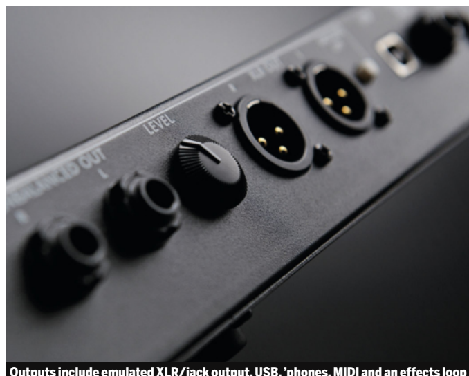
Outputs include emulated XLR/jack output, USB, 'phones, MIDI and an effects loop
