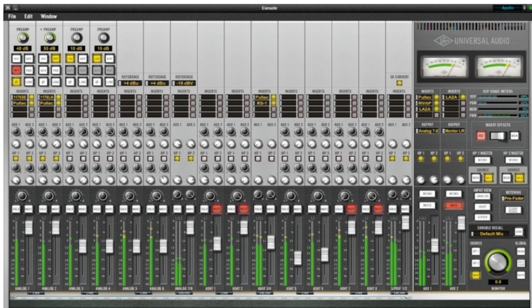
All of Apollo's front-panel hardware features can be controlled using the main software interface, Console
