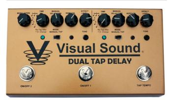
Like many other Visual Sound pedals, this is a two-in-one design, although with channel one's modulation control you can add in chorus too. Aside from that, the two delay channels are identical: maximum one-second delay time and controls for time division, delay time, repeats and effect level plus a manual/ tap switch and mini tone control. Three hefty footswitches operate each channel's on/off status (both can be used simultaneously) and the tap tempo.
