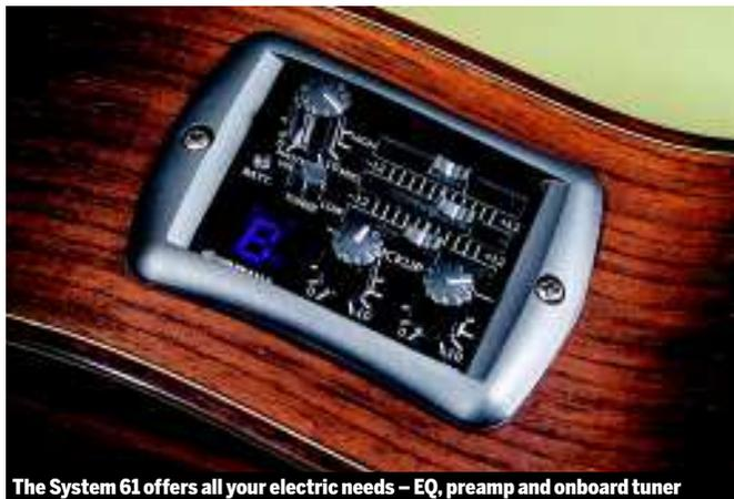
The System 61 offers all your electric needs – EQ, preamp and onboard tuner
