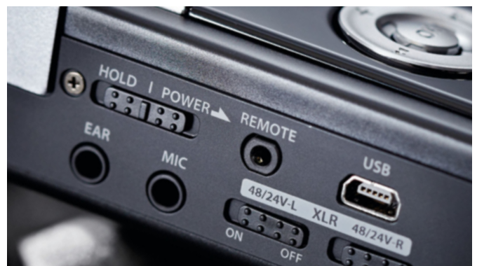
The LS-100 can be used as a USB audio interface and has phantom power for mics
