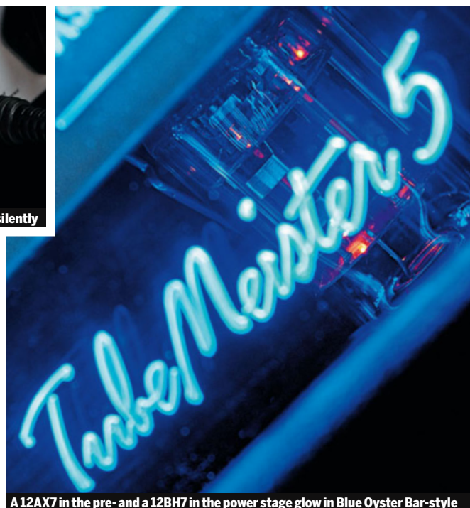
A 12AX7 in the pre- and a 12BH7 in the power stage glow in Blue Oyster Bar-style
